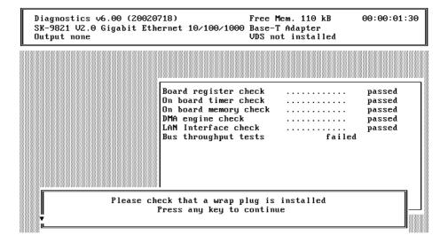
Figure 7. Typical error message from the diagnostics program
